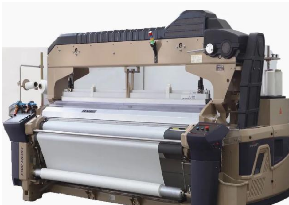
2.43-rasm. Suv tomchisi yordamida arqoq tashlovchi HAIJIA to‘quv dastgohi
