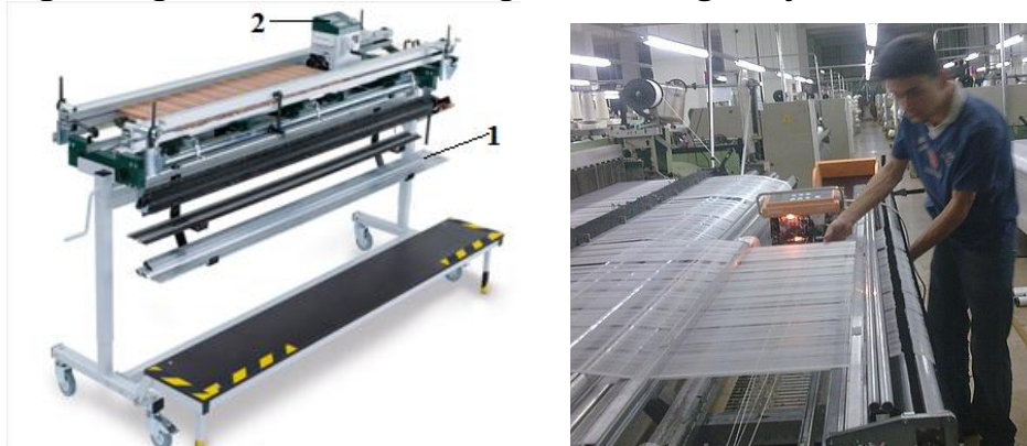
1.93-rasm. Bog‘lash mashinasi (2) va aravachasining (1) ko‘rinishi
