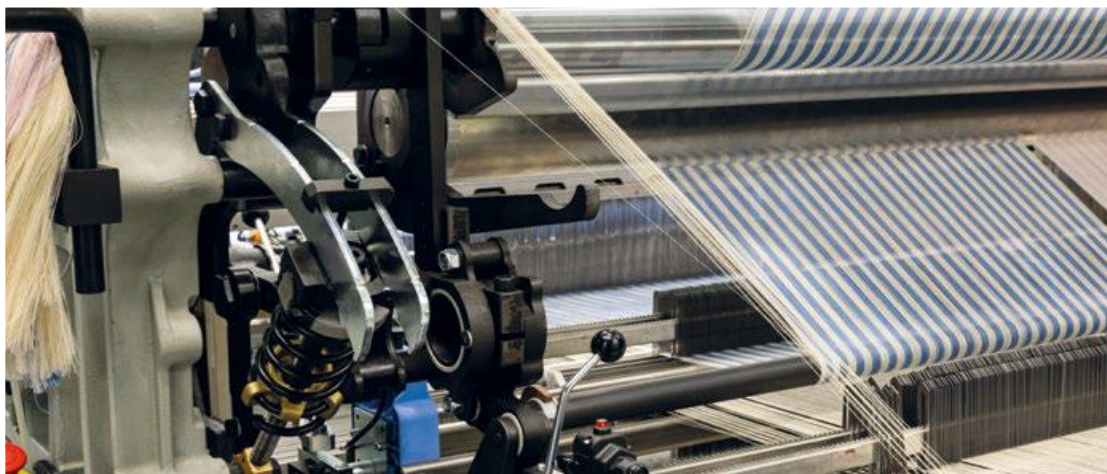
2.39-rasm. R9500 EVO Terry dastgohidagi tuk tanda ipi tarangligini nazorat qilish mexanizmi
