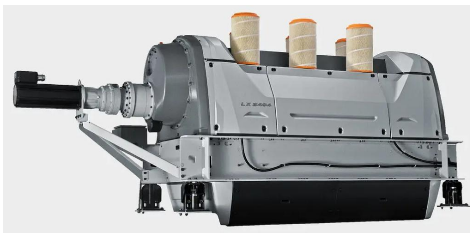
2.23-rasm. Gilam, baxmal va texnik to'qimalarga mo'ljallangan LX 2494 markadagi jakkard mexanizmi
